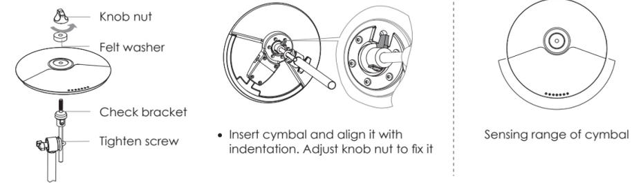
• Insert cymbal and align it with indentation. Adjust knob nut to fix it
