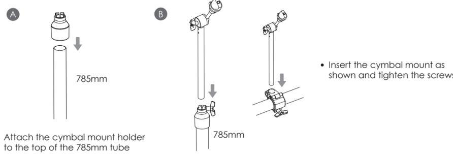
• Attach the cymbal mount holder to the top of the 785mm tube
