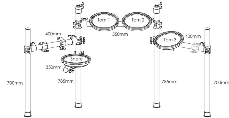
• According to above figure, to assemble the stand and pad in turn.
