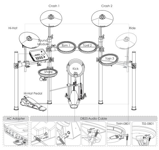
• To connect the jacks as shown in the figure, and using cable clip to organize the cables
