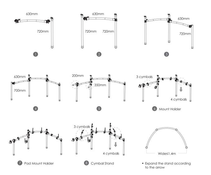
According to above figure, to assemble the stand and pad in turn.
